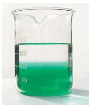
Figure 1.15 Diffusion within nickel(II) sulfate solution can take days to reach the stage shown on the right.
